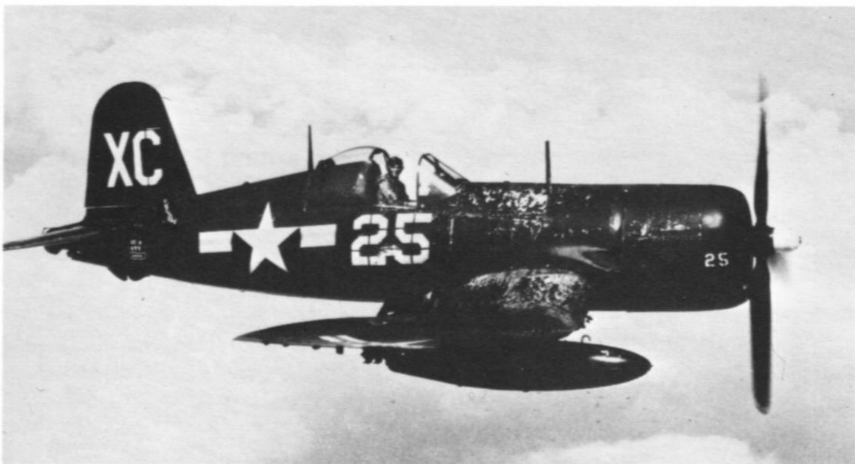
F4U-4, 96887, of VX-3 carries a standard Navy 150-gallon drop tank. Note the pattern of the split stenciling in White on the fuselage and rudder, also the heavily worn paint just forward of the cockpit and on the wing. This Corsair has the later-style blown canopy, c.1952. (Walt Ohlrich)
