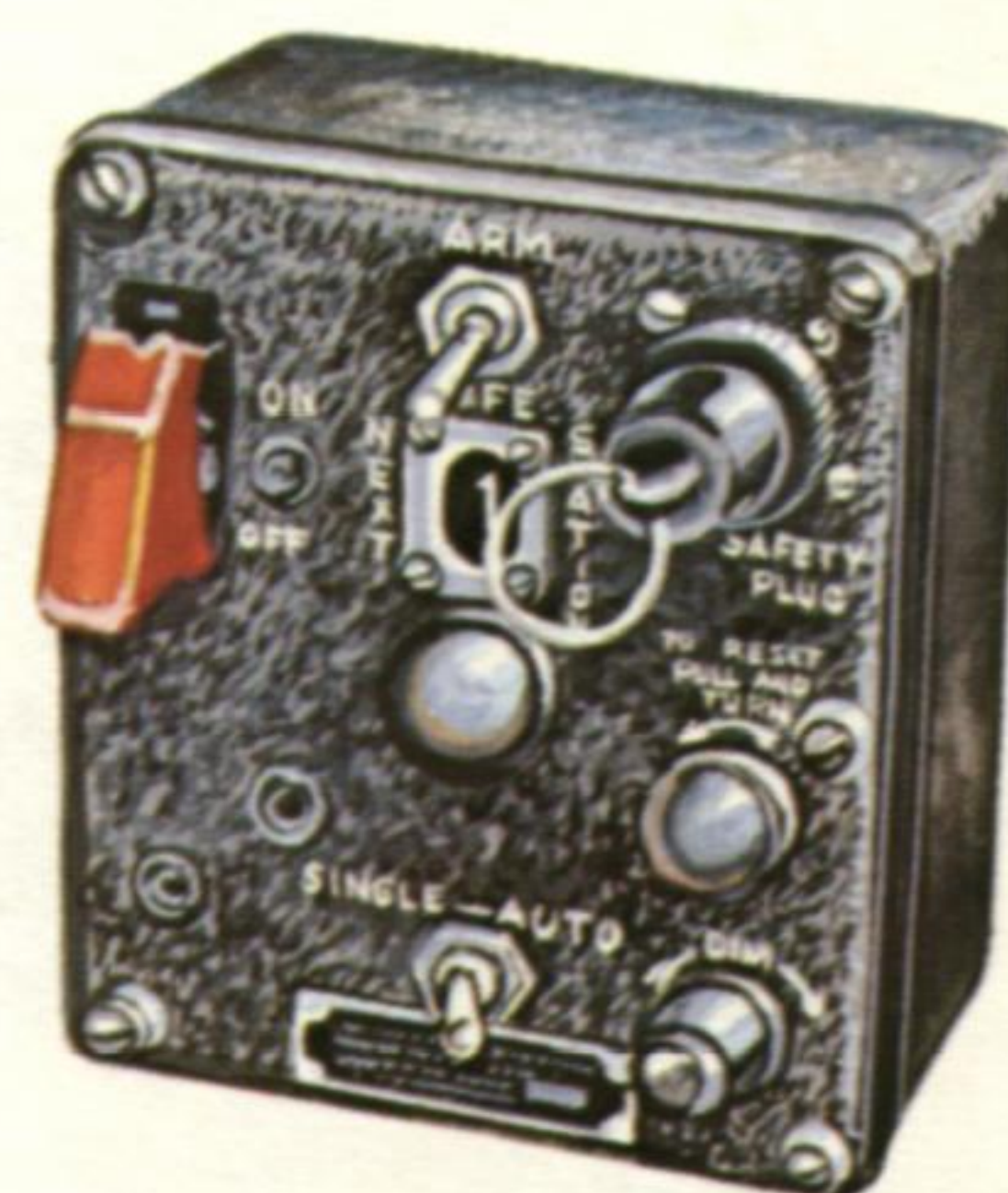
Rocket Station Distributor Box Installed on F4U-1/FG-1Ds
