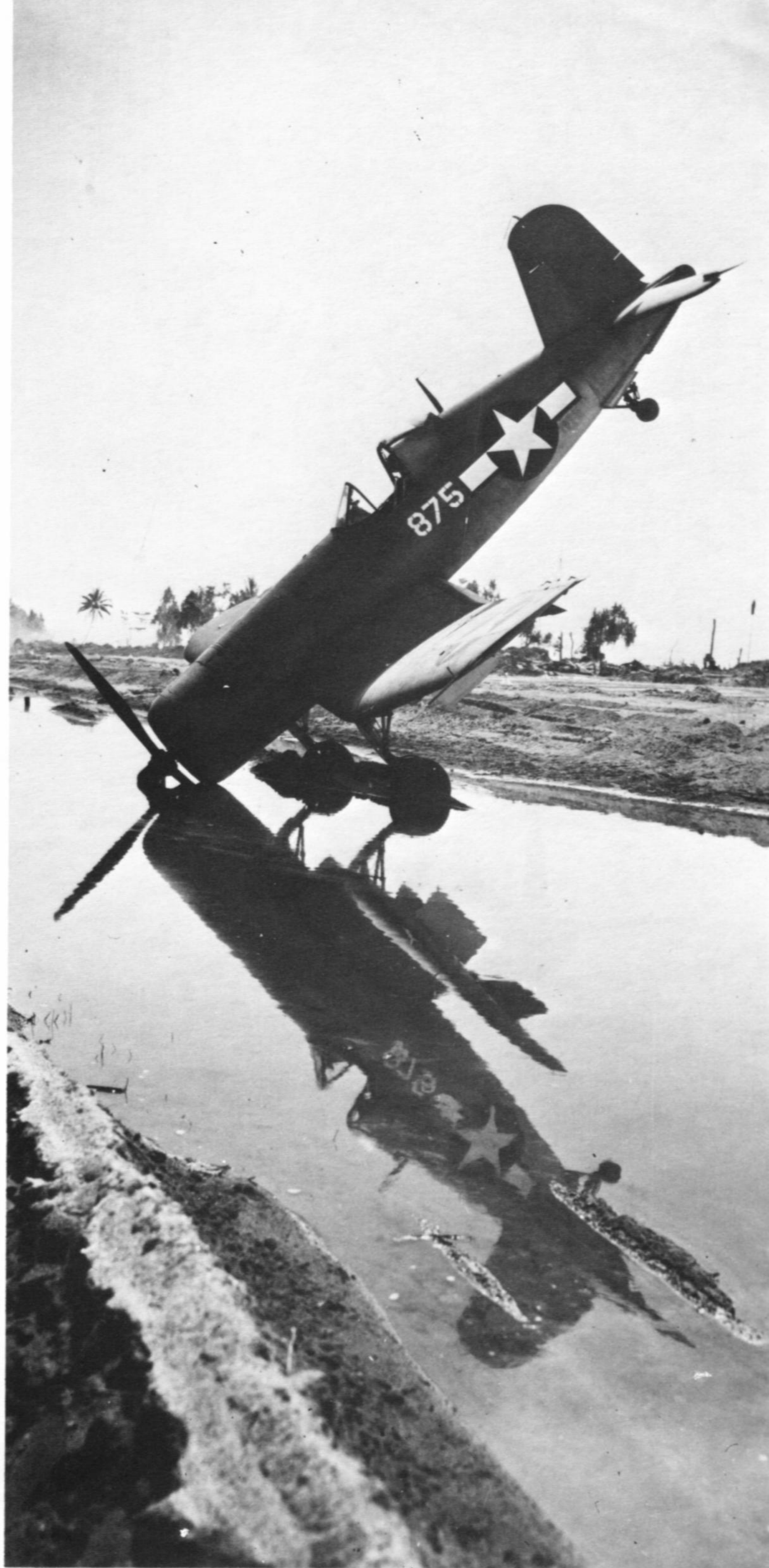
F4U-1A, 17875, of VMF-212 in a three-tone finish, skidded off Torokina Field during take-off. The pilot was uninjured and the Corsair needed only a new prop, 20 December 1943. (USMC)
