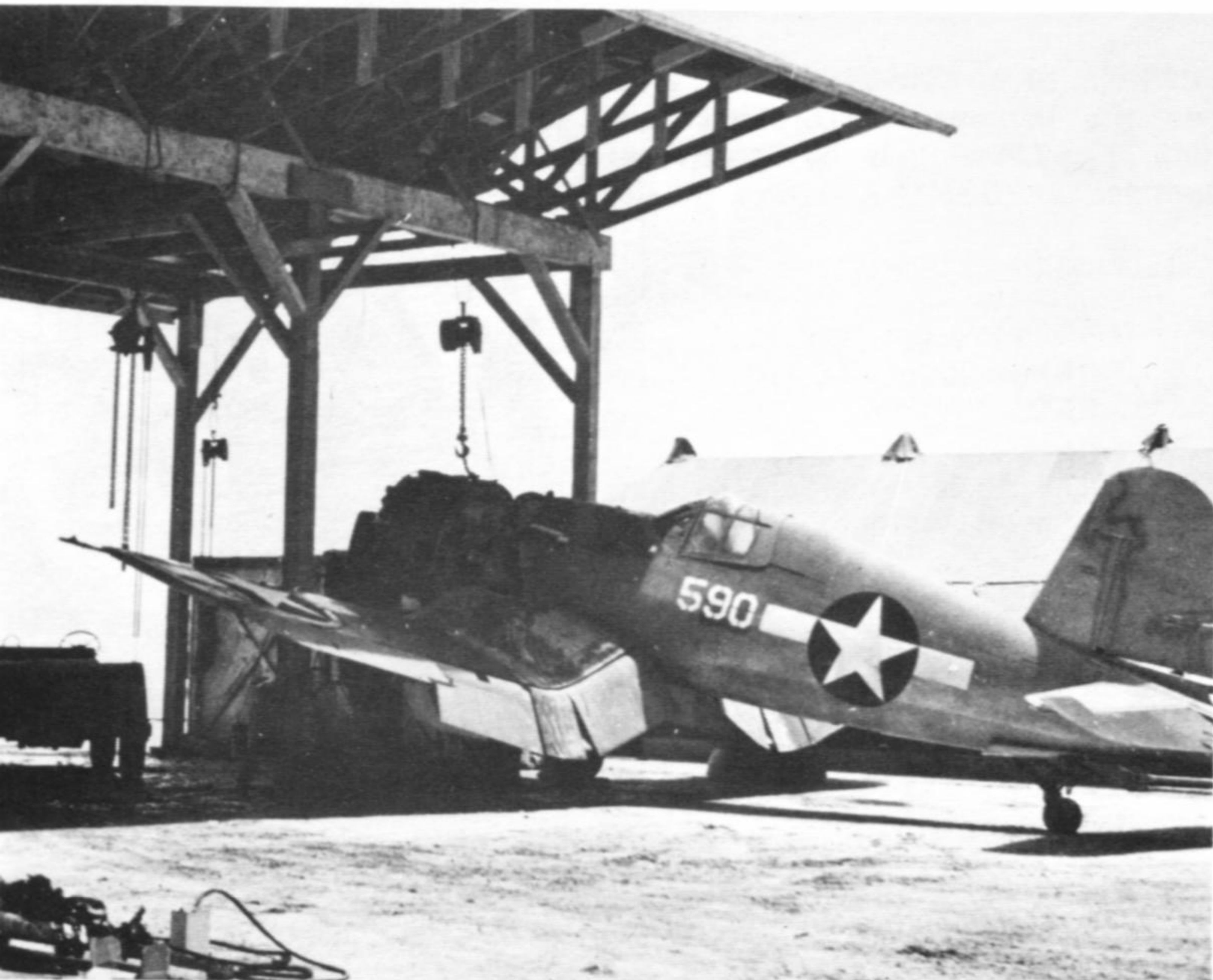
F4U-1, 17590 of VMF-223 during an engine change on Vella Lavella, 10 December 1943. The 590 split stenciled in white is taken from the last three digits of the aircraft Bureau Number (BuNo). The national insignia has been updated by having White bars added to the Blue roundel. (National Archives)
