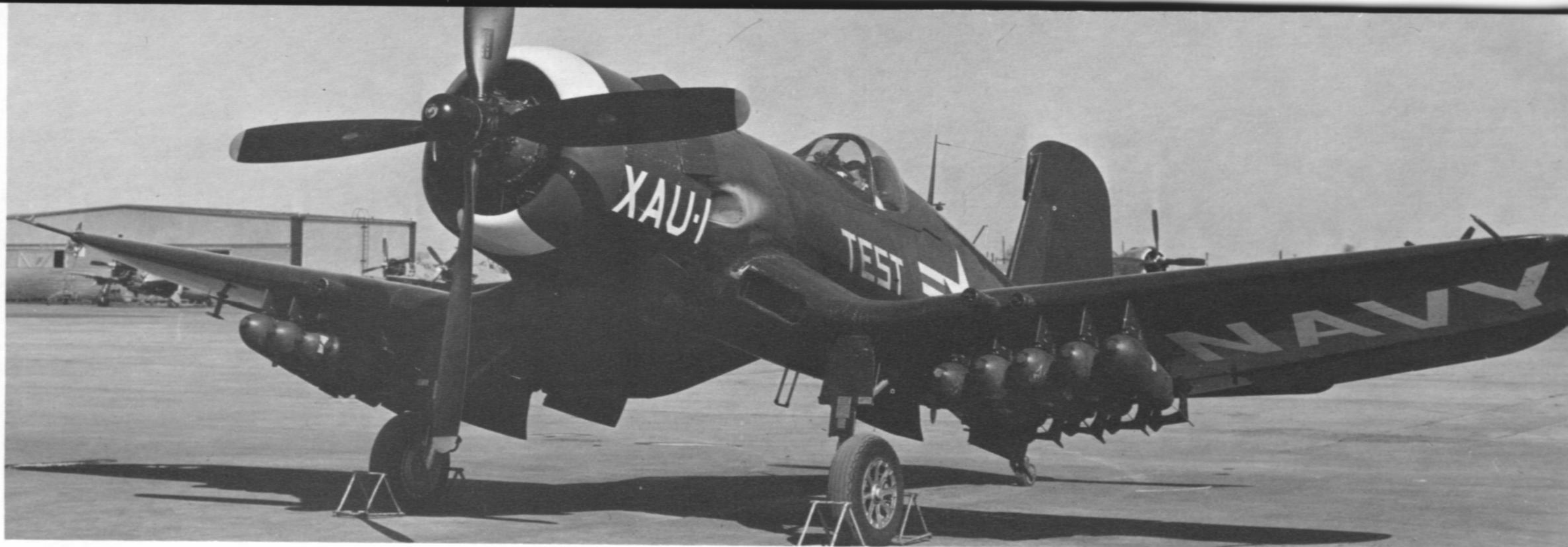
This F4U-5N, 124665, has been modified to become the XAU-1 (F4U-6). The cheek intakes were faired over and underwing racks to handle ten rockets or bombs were added. Designed as a close support aircraft it was powered by a P&W R2800-83W engine. Overall glossy Sea Blue, the cowl is segmented with White and Red panels. 18 March 1952. (Chance Vought)
