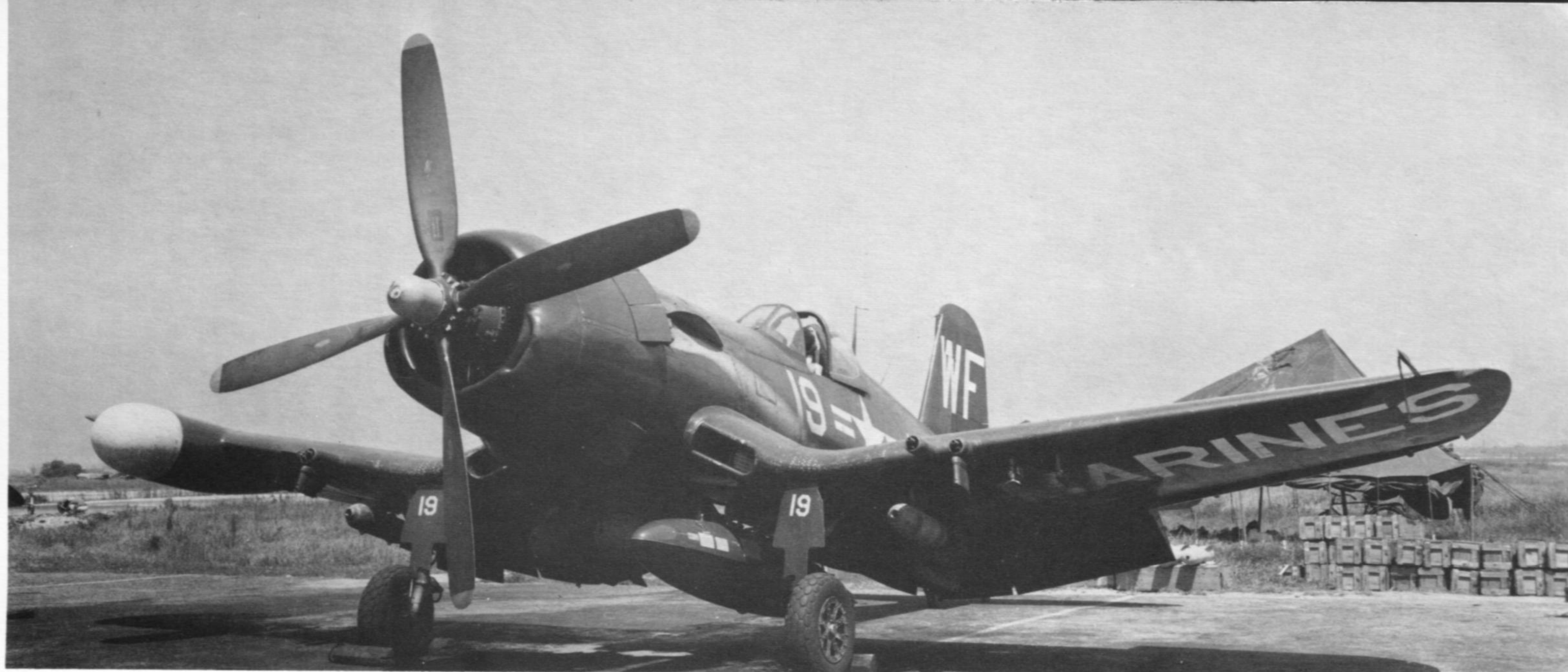
F4U-5N Nightfighter, 123183, of VMF(N)-513 loaded with 500 lb. fire bombs and 265 lb. fragmentation bombs ready to fly to its Korean target from a base in Japan. The Flying Nightmares flew Corsairs throughout the Korean War, November 1950. (USMC)
