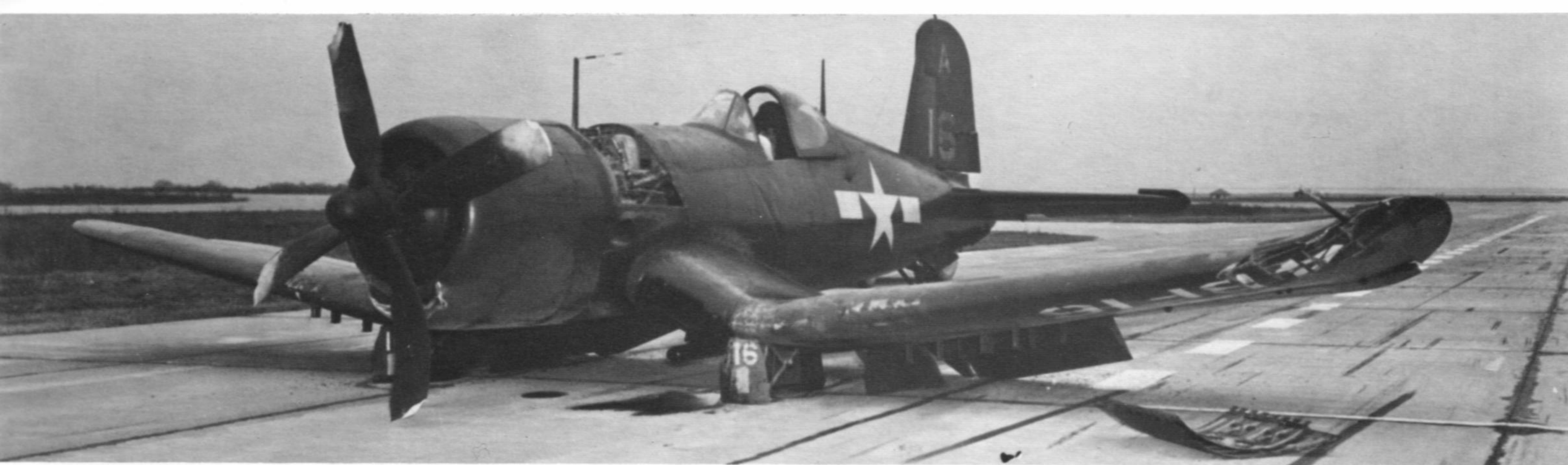
F4U-4, 80960, No. 16 of VBF-4 slid to a grinding halt at NAS Chincoteague, VA. This bellied-in Corsair has its tailwheel extended while the front of the aircraft seems to be resting on its dive brake fairings and landing gear doors. Rudder markings in Yellow, all others are White. 26 January 1946. (National Archives)
