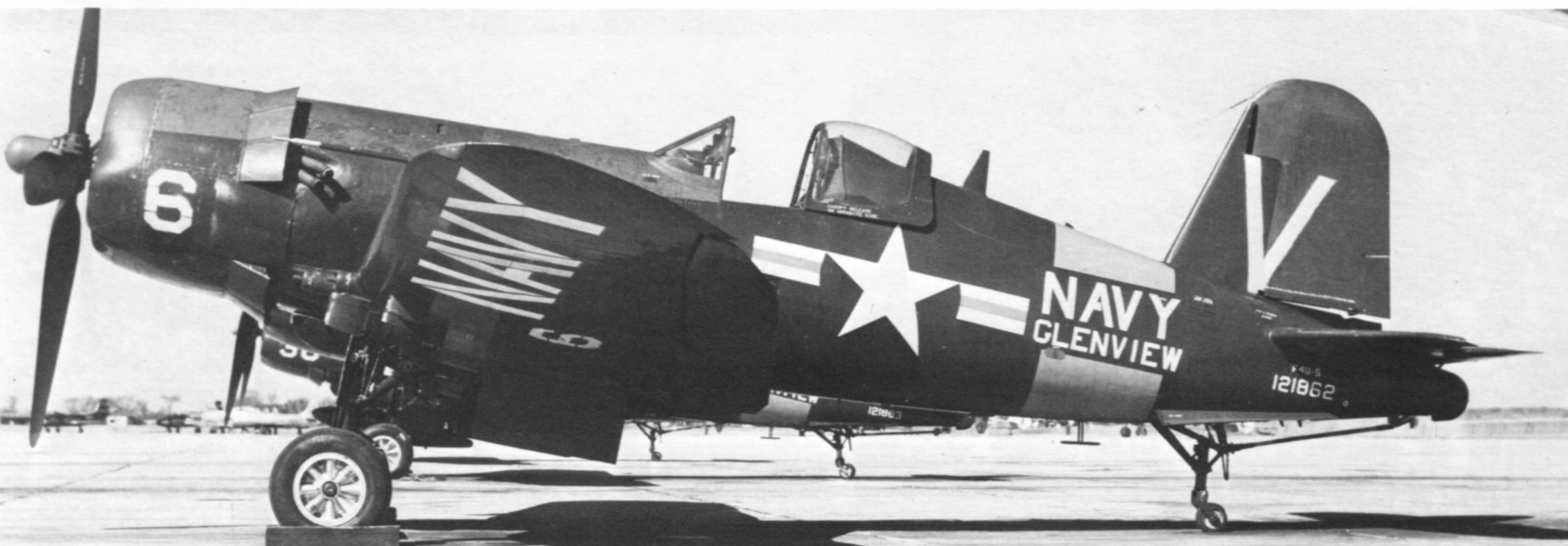
F4U-5, 121862, No. 6 carries the international Orange fuselage band indicating reserve status. The matte Sea Blue anti-glare panel can be seen very clearly on this machine. 1954. (Eric Luhdahl)
