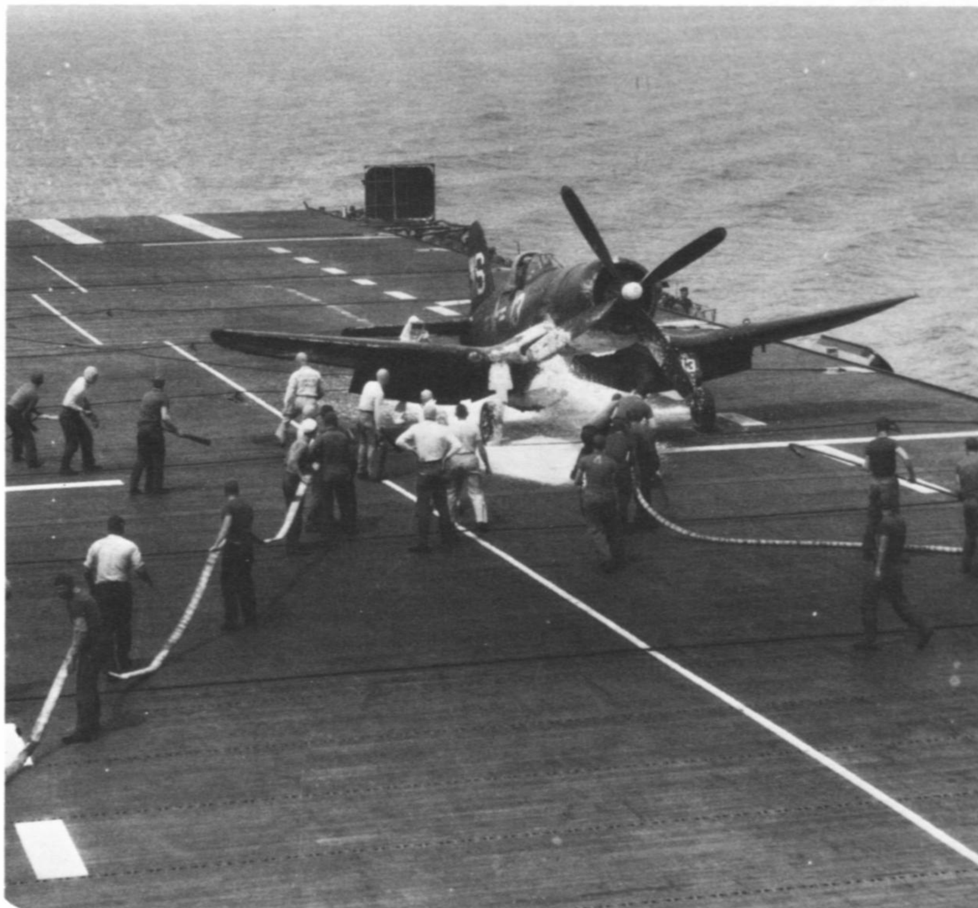
A loose gas cap on its drop tank was the cause of this fire as F4U-4, 96821, was recovering on board Sicily off Korea. This machine, No. 13, belongs to VMF-323 Deathrattlers. 11 June 1951. (USMC)
