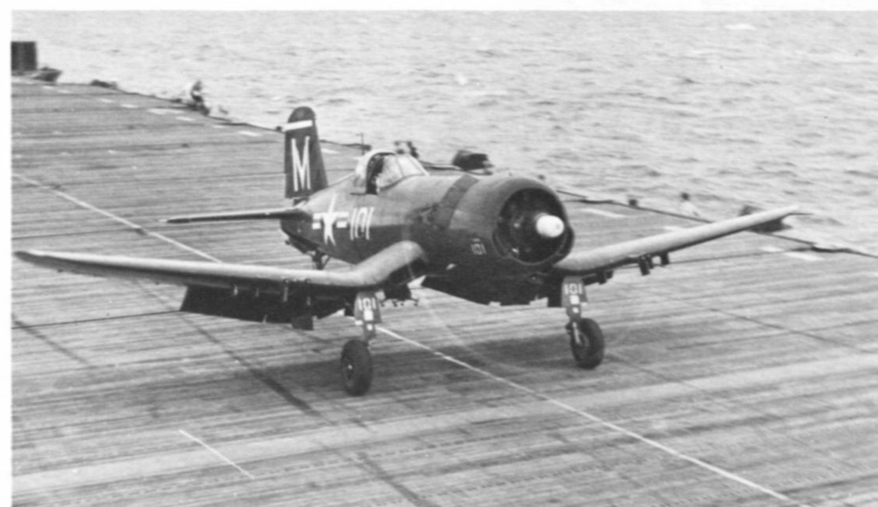
F4U-5 of VF-21 lands on board USS Wright during arresting gear test conducted off the Florida coast. The tail stripe is White. 3 November 1948. (Cdr. R.E. Bennett, USNR)
